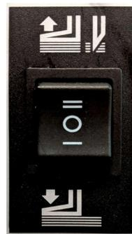
3. Flip the main toggle switch upwards to the ON position and the control panel display will come to life. If it does not, go back to step #2. Before operating the cutter, wait for the Back Gauge to calibrate and check if the blade and paper clamp are in the standby position which should be all the way up. If not, press UP (=) on paper clamp up/down control until both have retracted after which you are able to proceed to using the cutter.
