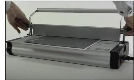
6) Set the pressure bar directly on the strip and make sure it locks firmly in place. Notice the hot knife lever's position should be exactly where it is for steps 1-6.
