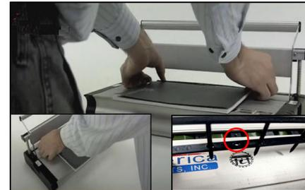
5) Carefully set your document on the binding shelf making sure the locating pin hole on the strip is properly positioned along with the locating pin on the machine.
