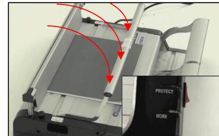
7) Carefully set the hot knife lever down and wait a few seconds until the Protect Indicator illuminates. **IMPORTANT!!! NEVER forcefully push the hot knife lever down as it may cause serious damage to the hot knife strip. Gently set it down and allow it to move along with the machine's cutting action.**
