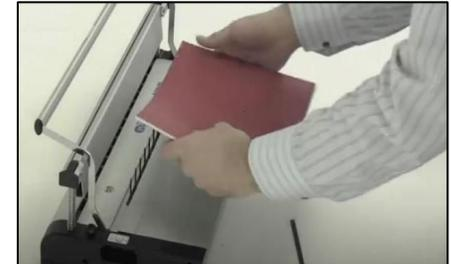
4) Position the strip on the binding channel for easier insertion of your documents.
