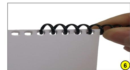
6. Manually insert the coil into the first 4 or 5 holes as shown.
