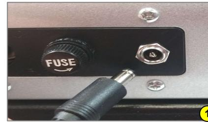
1. Plug the male connectors (power cord & foot pedal) into the receptacle at the back of the machine then connect the power cord into an electrical outlet.
