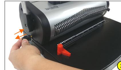
3. Adjust depth margin from 2.5mm to 6.5mm. This controls how far or how close you want the holes to be in relation to the edge of the document.
