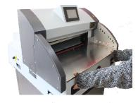
Press 2 cut buttons simultaneously
