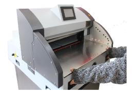
Press 2 cut buttons simultaneously
