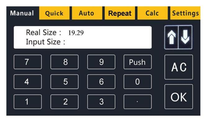
On start-up, the cutter will default to 19.29" as denoted by the **Real Size** value which essentially is the current size adjustment. To manually program a cut size, simply do the following:
