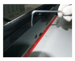
2. Loosen the seven M6 fasten screws and adjust the screws on the blade carrier until the blade cuts into the cutting stick by about 0.3-0.5mm.
