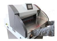
Press 2 cut buttons simultaneously
