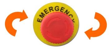
2. In order to operate the cutter, make sure the emergency stop switch is in the ON position by moving the knob according to the direction of the arrows (clockwise). Simply push down on the knob In the event of any emergency where you need to immediately cut power to the cutter.
