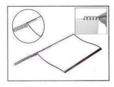
4. Manually insert the coil into the first 4 or 5 holes as shown. Do this for all holes for models without a coil inserting roller (Procoil-53).
