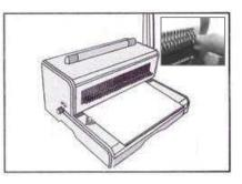
2. Adjust ruler guide according to the size of your document & disengage pins that would punch off the edge of the document by pulling them towards you.
