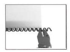
6. Use the handheld coil crimper pliers to crimp the ends to keep the document from unbinding.
