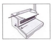
Press the coil inserter roller switch to the ON position then grasp the document and gently press against the coil against the roller.
