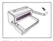
3. Pull punch handle downwards to punch holes on the document then retract to original position.
